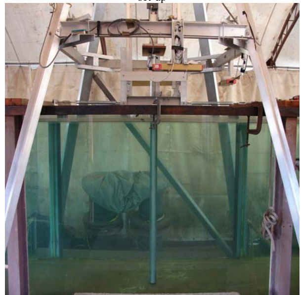
Figure 7: Side view of Stratified Flow Channel. The vertical cylinder is the test cylinder.
